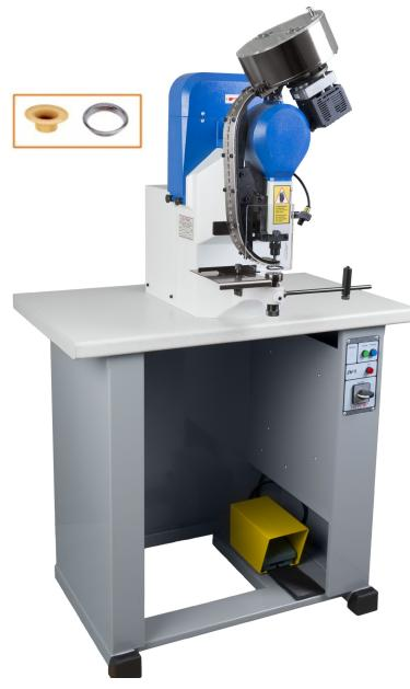
Automatically sets grommet and washers and punches through most material in one stroke
