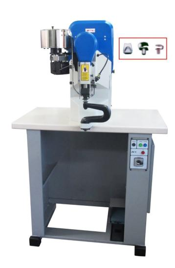
Automatically Feed Hook machine that will punch & set hooks into leather or similar material.
